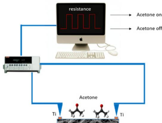
Figure 2: Chemiresistive sensor testing system.
