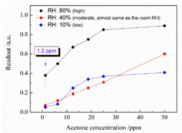
Figure 3: Sensor performance under different RH levels.
