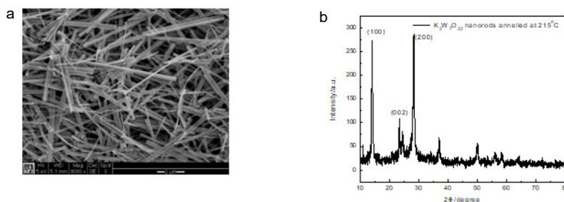
**Figure 1:** (a) SEM images of  $K_2W_7O_{22}$  nanorods synthesized at 215°C. (b) XRD pattern of synthesized  $K_2W_7O_{22}$  nanorods at 215°C.
