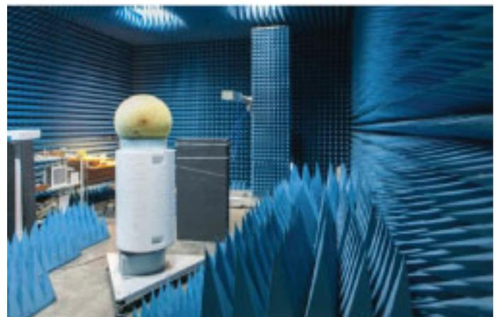
**Figure 3.** Illustrates Radio frequency anechoic chamber used for the research.<sup>11</sup> Image Credit: ITMO University
