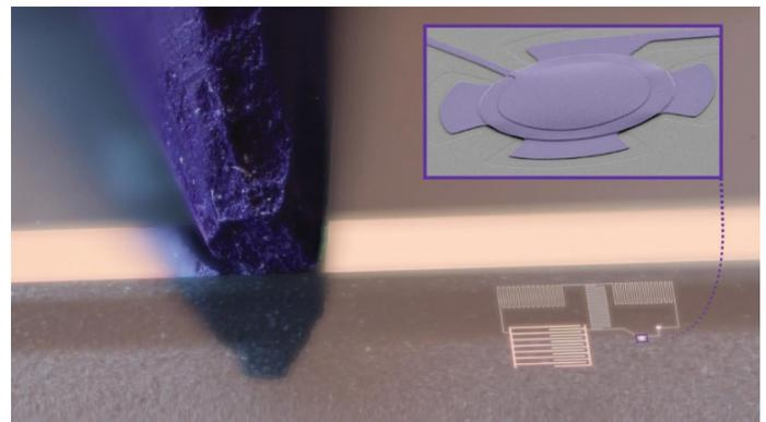
**Figure 1.** Illustrates the chip used in the experiment to couple a microwave cavity to micrometer size drum.<sup>7</sup> Image Credit: N. R. Bernier and L. D. Tóth (EPFL).
