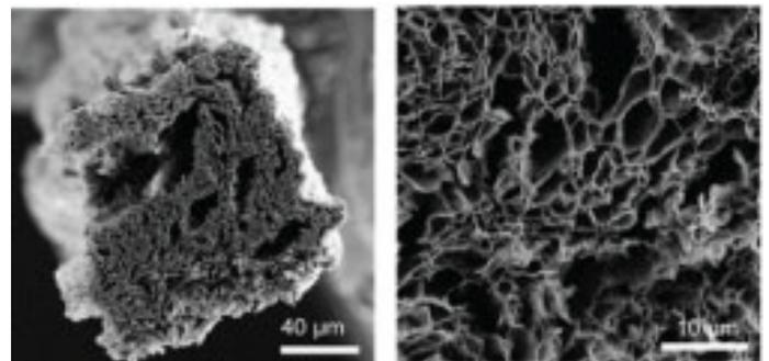
**Figure 2.** Illustrates scanning electron microscopy of a graphene fiber constructed from microwave reduced graphene oxide.<sup>9</sup> Image Credit: Jieun Yang, Damien Voiry and Jacob Kupferberg
