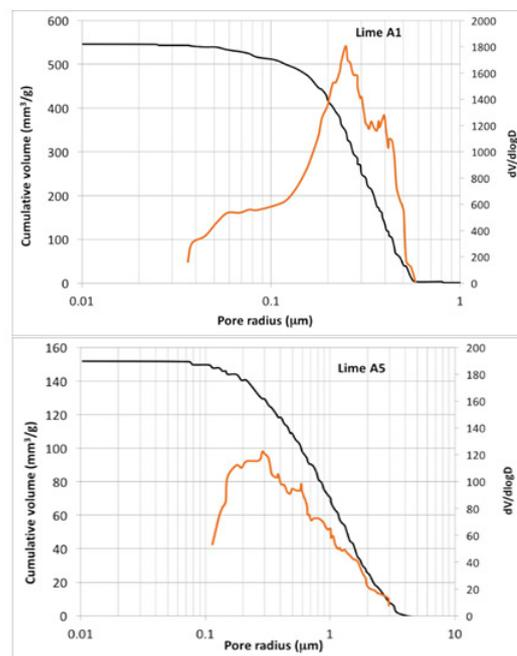
**Figure 4:** Cumulative and differential pore size distribution from Hg porosimeter analysis for sample A1 and A5.
