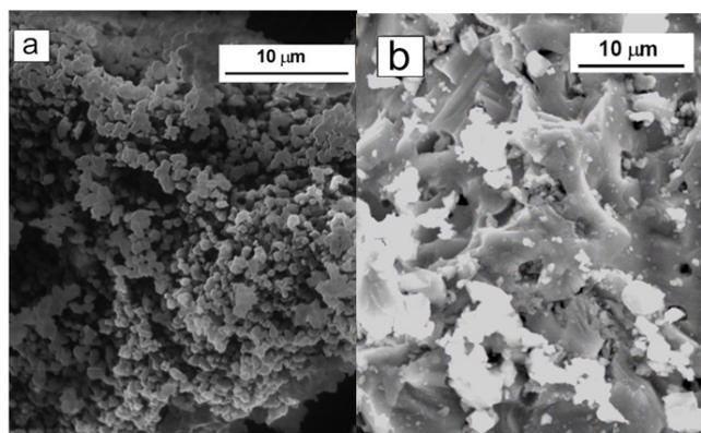
**Figure 3:** Morphological SEM image of lime A1 (a) and A5 (b) obtained for decomposition of limestone A at 980 °C and 1300 °C respectively.
