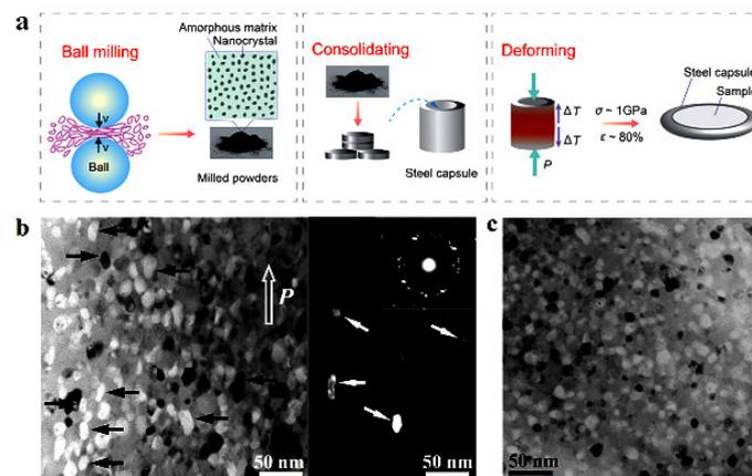
**Figure 2:** Fabrication of bulk anisotropic  $\text{SmCo}_7/\text{Fe}(\text{Co})$  nanocomposite magnets containing ~ 28 wt.%  $\text{Fe}(\text{Co})$ . a) Schematic representation of the method. b) and c) TEM characterization of the nanocomposites along (b) and perpendicular to (c) the pressure direction.
