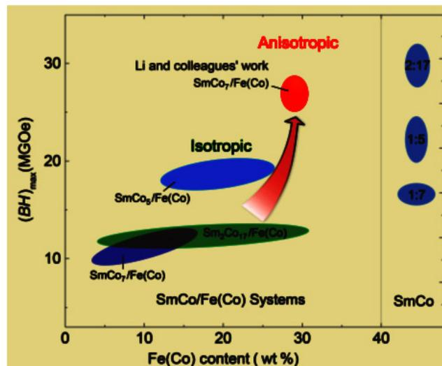
**Figure 1:** Comparison of energy products for different bulk  $\text{SmCo}/\text{Fe}(\text{Co})$  nanocomposite systems (right panel) and their corresponding pure  $\text{SmCo}_7$  (1:7),  $\text{SmCo}_5$  (1:5), or  $\text{Sm}_2(\text{Co,Fe,Cu,Zr})_{17}$  (2:17) rare-earth magnet (left panel).
