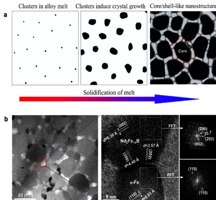
**Figure 4:** 3D self-assembly of core/shell-like hybrid nanostructures. a) Schematic representation of the self-assembly process. b) TEM characterization of the core/shell-like nanostructure with  $\text{Nd}_2\text{Fe}_{14}\text{B}$  core and  $\alpha\text{-Fe}$  shell.
