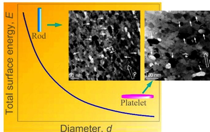
**Figure 3:** Schematic of the total surface energy  $E$  of an oriented nanocrystal (along the normal direction of low-surface-energy faces) as a function of crystal diameter. The insets show the bright-field TEM images for hard-phase nanograins with a rod or disc shape in the magnets yielded at different deformation temperatures.
